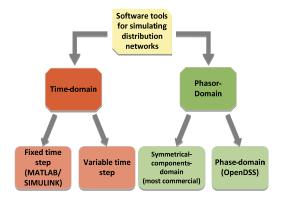
Software tools based on time-domain solutions simulate the power system network by solving differential equations that describe all power system components. Although these simulation tools provide the ability to integrate DG control schemes in a very straightforward manner, they cannot be used for the simulation of extended networks, due to the prohibitive execution times.
